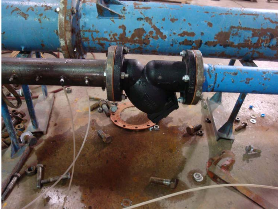
Figure 2. 4-inch strainer installation (Competitor strainer shown).
