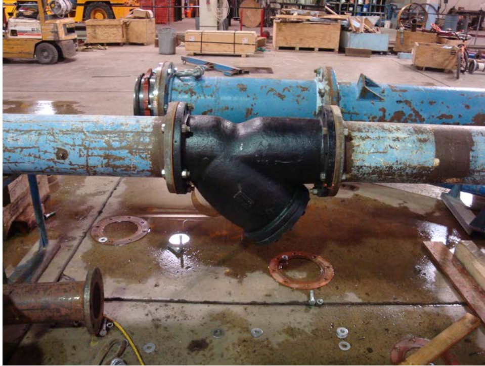
Figure 2. 10-inch strainer installation (Competitor strainer shown).
