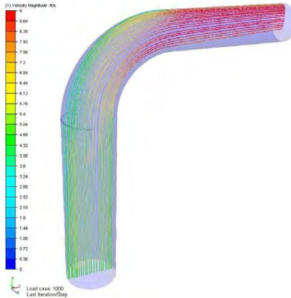
**Figure 6.** Fluid particle traces shown for the non-SDF analysis. Note the fluid separation around the elbow. This separation region propagates well downstream.
