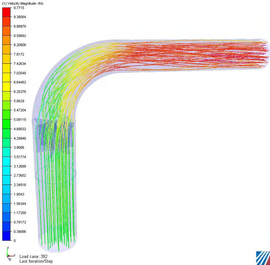
**Figure 8.** Particle traces showing the effectiveness of the SDF.
