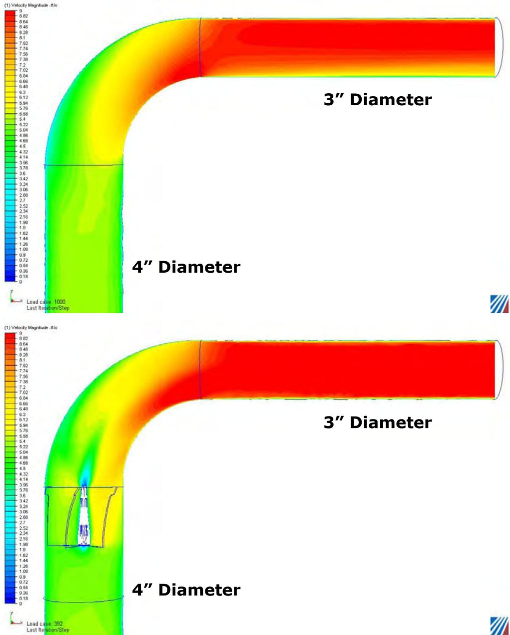
**Figure 2.** Cut-surface showing velocity contours through the reducing elbow.
