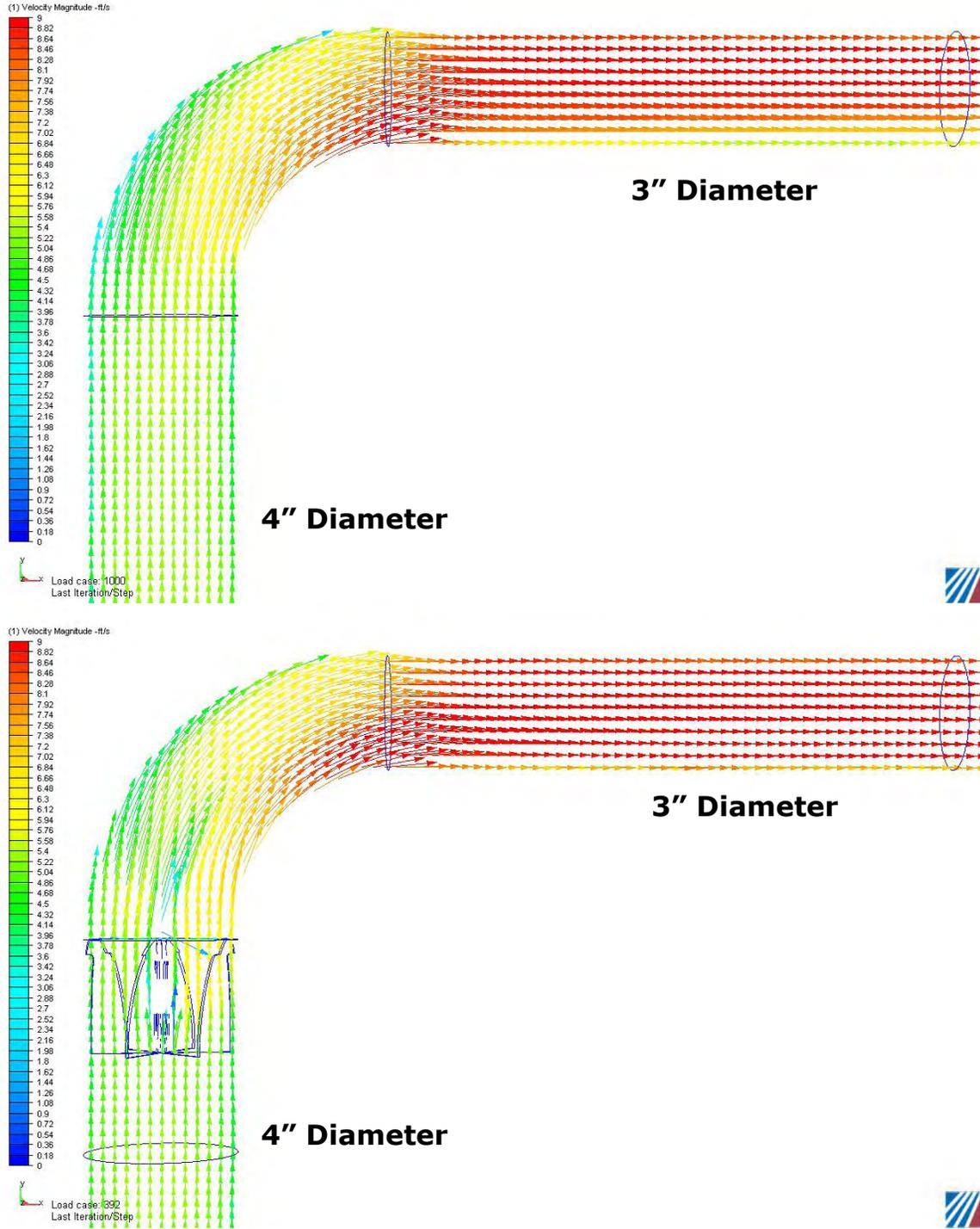
Figure 3. Cut-surface showing velocity vectors through the reducing elbow.
