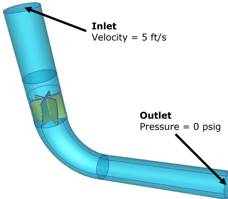
**Figure 1.** CFdesign analysis setup conditions.
