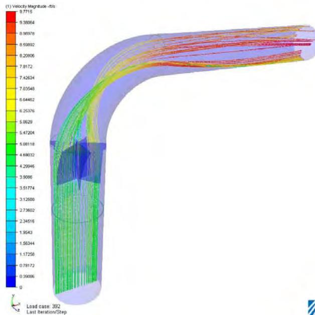
**Figure 7.** Induced swirl caused by the SDF as shown with particle traces.
