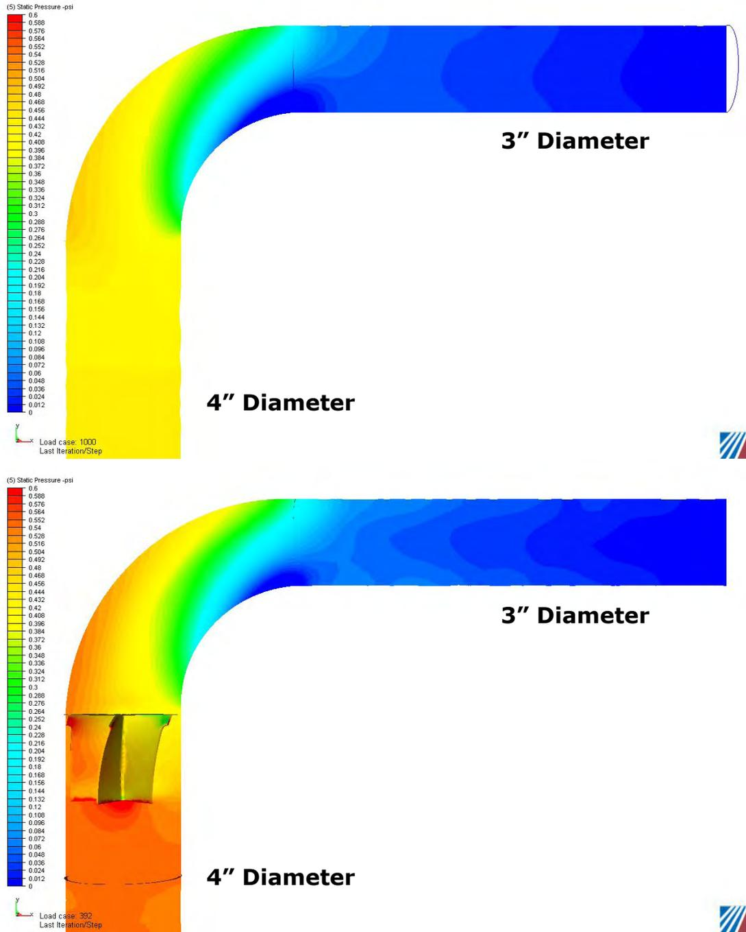
**Figure 5.** Cut-surface showing pressure gradients through the elbow.
