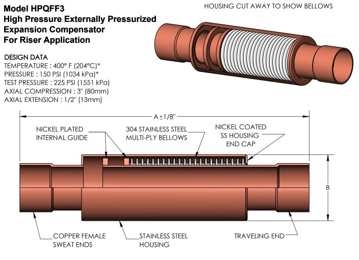
This expansion joint is designed for use in riser applications and axial movement only. Consult Metraflex for guiding and anchoring of pipe in riser application. For horizontal runs, the guiding and anchoring recommendations of the Expansion Joint Manufacturers Association is to be followed.
