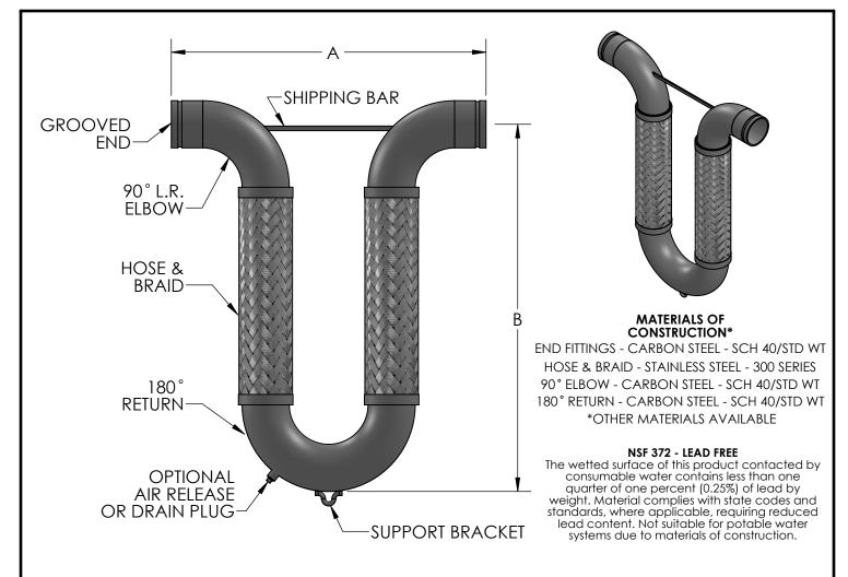
NOTE: METRALOOPS 2" AND LARGER INSTALLED IN ANY ORIENTATION OTHER THAN HANGING DOWN MUST HAVE THE 180° RETURN SUPPORTED. (SEE INSTALLATION INSTRUCTIONS.)
