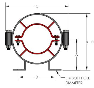
SPIDER SPACERS CENTER PIPE IN HOUSING AND ARE SIZED TO ALLOW INSULATION TO BE PACKED AROUND PIPE SPLIT HOUSING FOR EASY INSTALLATION MVMT · FEET CAN BE **BOLTED OR** WELDED TO DIRECTION OF - 11-**STRUCTURE** PIPE MOVEMENT \*EXTENDED SPIDER GUIDES ARE AVAILABLE. CONTACT METRAFLEX FOR OPTIONS. LEADING EDGE OF SPIDER SET HALFWAY
