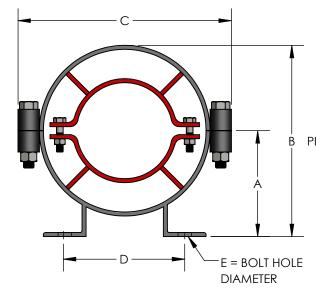
SPIDER SPACERS CENTER-PIPE IN HOUSING AND ARE SIZED TO ALLOW INSULATION TO BE PACKED AROUND PIPE SPLIT HOUSING FOR EASY INSTALLATION MVMT . FEET CAN BE **BOLTED OR DIRECTION OF WELDED TO** STRUCTURE PIPE MOVEMENT \*EXTENDED SPIDER GUIDES ARE AVAILABLE. CONTACT METRAFLEX FOR OPTIONS. LEADING EDGE OF -SPIDER SET HALFWAY
