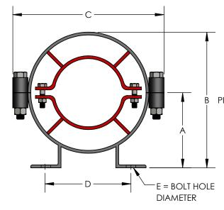
SPIDER SPACERS CENTER PIPE IN HOUSING AND ARE SIZED TO ALLOW INSULATION TO BE PACKED AROUND PIPE SPLIT HOUSING FOR EASY INSTALLATION MVMT · FEET CAN BE **BOLTED OR** WELDED TO DIRECTION OF **STRUCTURE** PIPE MOVEMENT \*EXTENDED SPIDER GUIDES ARE AVAILABLE. CONTACT METRAFLEX FOR OPTIONS. LEADING EDGE OF SPIDER SET HALFWAY
