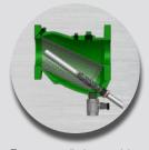
To ensure all the particles captured are blown out during the blow down process, slowly draw the magnet(s) out of the drywell and stop when you see the red line.
