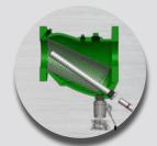
Open the valve and blow down for 3 to 5 seconds and at the same time pull the magnet the rest of the way out. Then shut the blow down valve. Re-insert the magnet.
