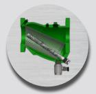
The magnets are constantly collecting magnetic debris while at the same time larger foreign materials are being captured in the perforated stainless steel screen.
