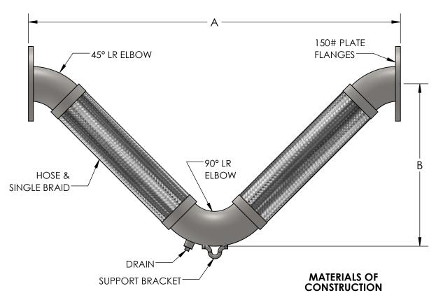
END FITTINGS - CARBON STEEL - SCH 40/STD WT HOSE & BRAID - STAINLESS STEEL - 300 SERIES ELBOWS - CARBON STEEL - SCH 40/STD WT
