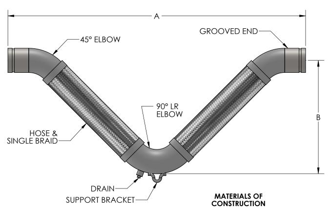
END FITTINGS - CARBON STEEL - SCH 40/STD WT HOSE & BRAID - STAINLESS STEEL - 300 SERIES ELBOWS - CARBON STEEL - SCH 40/STD WT
