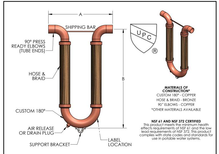
NOTE: METRALOOPS 2" AND LARGER INSTALLED IN ANY ORIENTATION OTHER THAN HANGING DOWN MUST HAVE THE 180° RETURN SUPPORTED. (SEE INSTALLATION INSTRUCTIONS.)
