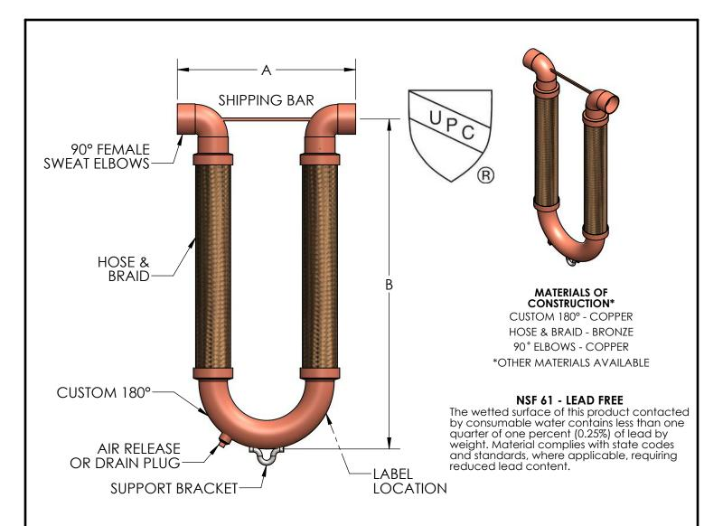
NOTE: METRALOOPS 2" AND LARGER INSTALLED IN ANY ORIENTATION OTHER THAN HANGING DOWN MUST HAVE THE 180° RETURN SUPPORTED. (SEE INSTALLATION INSTRUCTIONS.)
