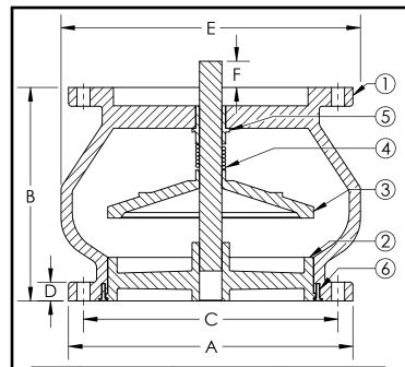
MAX NON-SHOCK WORKING PSI TEMPERATURE PSI\* 150°F 300 200°F 280 \*Sizes 14" and Up 12" - 400/370PSI
