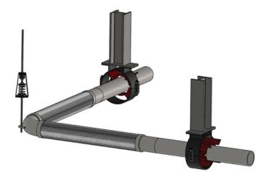
For larger pipe runs or movements greater than 4". Support is required for the 90° return fitting. Support can be either a spring hanger from above or a slide support from below.
