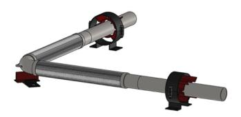
For horizontal pipe runs of 3" pipe and smaller with 4" movement or less, no additional support for the 90° return fitting is required.
