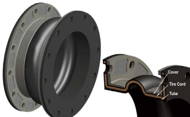
Figure 2C: Wide Arch Non-Metallic Reinforced Type Expansion Joint
