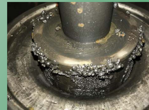
Accumulation of sludge within ECM Pump
