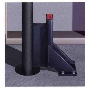
Floor and ceiling guides are designed so there is no metal-to-metal contact between T-slide and guide channel. Special non-metallic "quiet-slide" insert eliminates noise. Rugged construction will last the life of your piping system.
