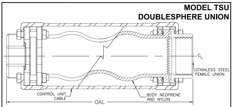
THIS FLEXIBLE JOINT SHOULD BE INSTALLED TO THE LENGTH SHOWN ON THIS DRAWING. THE CONTROL UNIT CABLES SHOULD BE REMOVED FOR THE INSTALLATION OF THE UNION ENDS. AFTER INSTALLATION THE CONTROL UNIT CABLES SHOULD BE REINSTALLED TO PREVENT MOVEMENT PAST DESIGN LIMITS. THIS PRODUCT IS NOT INTENDED FOR TORSION.
