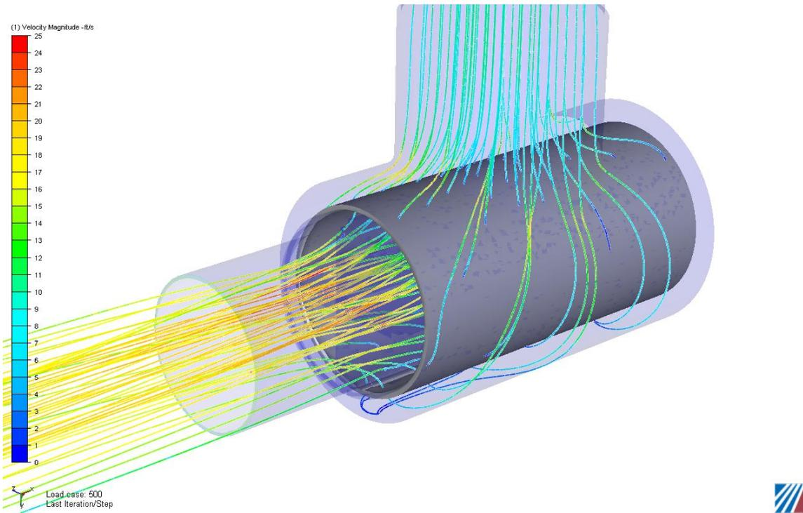
Figure 14. Fluid particle traces. (Cylindrical diffuser)
