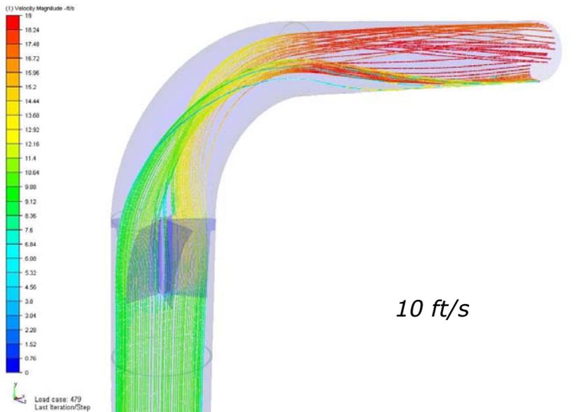
**Figure 7.** Fluid particle traces shown for the 10 ft/s flow rate.
