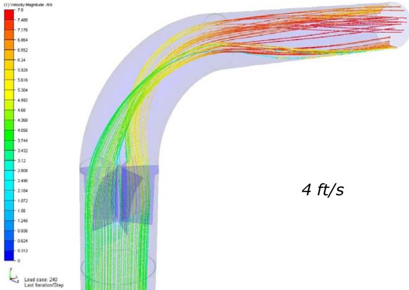
**Figure 6.** Fluid particle traces shown for the 4 ft/s flow rate.
