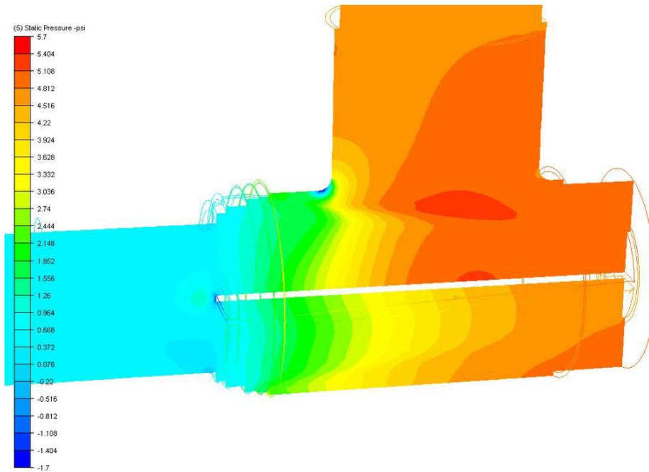
**Figure 4.** Cut-surface showing pressure data. (Conical diffuser, 10 ft/s)
