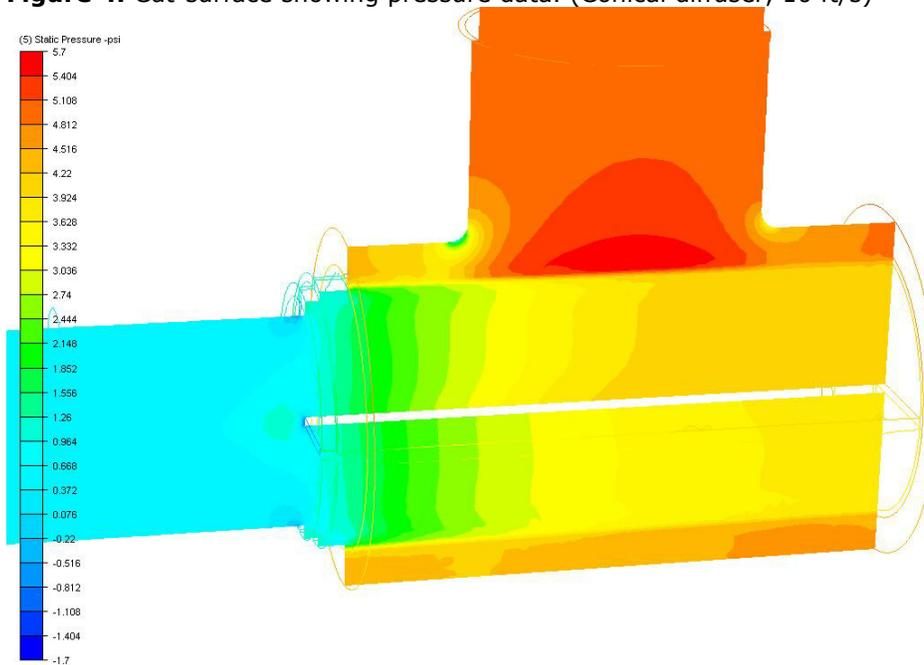
**Figure 5.** Cut-surface showing pressure data. (Cylindrical diffuser, 10 ft/s)
