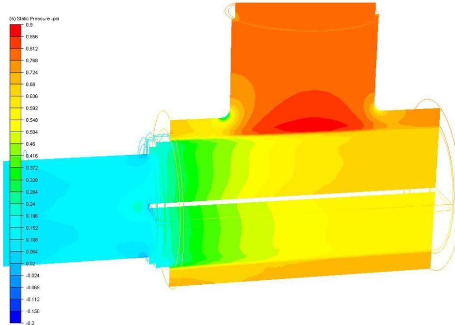
**Figure 3.** Cut-surface showing pressure data. (Cylindrical diffuser, 4 ft/s)
