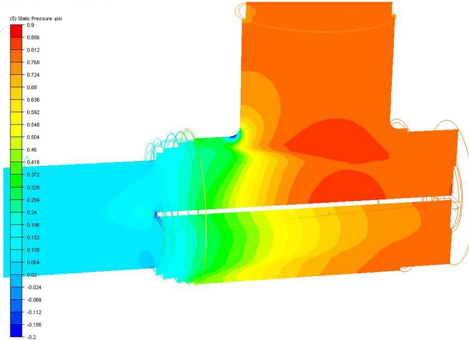
**Figure 2.** Cut-surface showing pressure data. (Conical diffuser, 4 ft/s)
