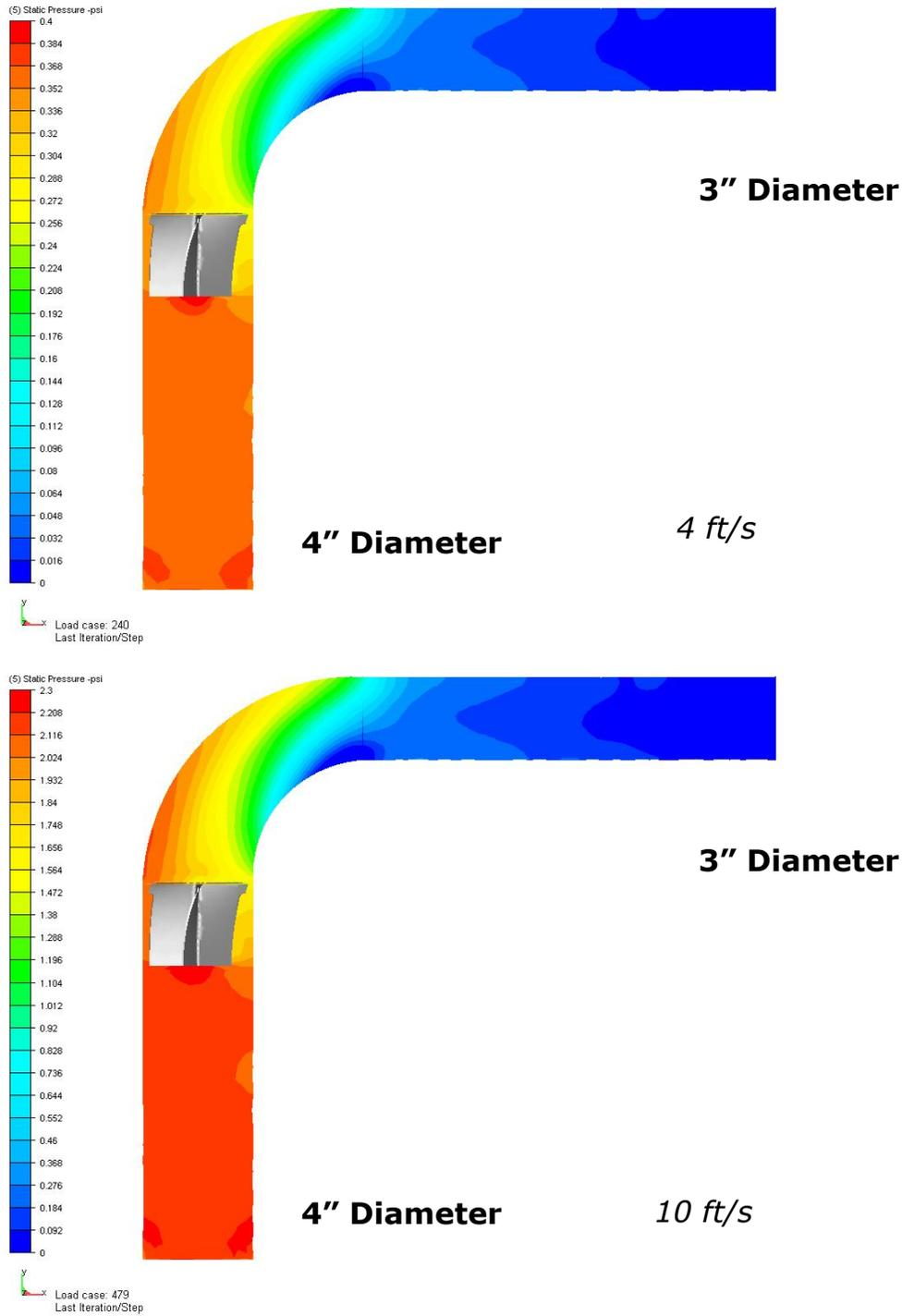
Figure 5. Cut-surface showing pressure gradients through the elbow.
