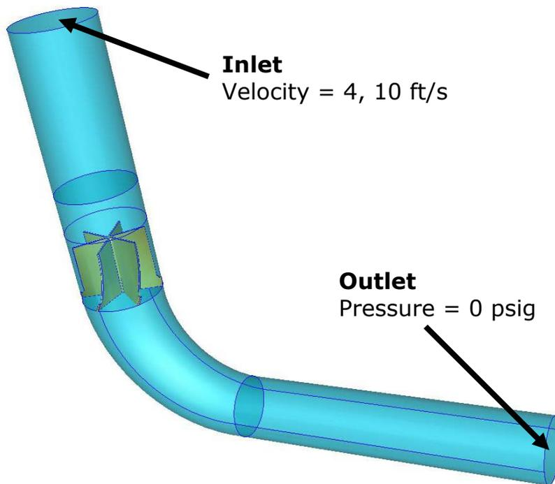
**Figure 1.** CFdesign analysis setup conditions.
