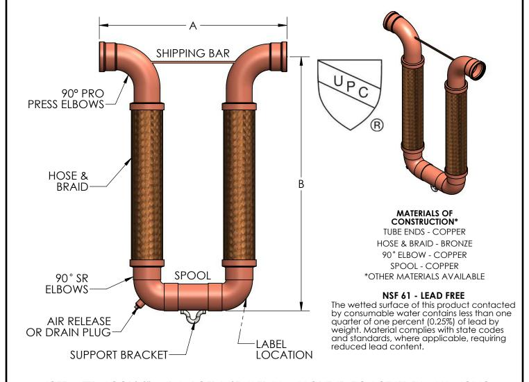
NOTE: METRALOOPS 2" AND LARGER INSTALLED IN ANY ORIENTATION OTHER THAN HANGING DOWN <u>MUST</u> HAVE THE 180° RETURN SUPPORTED. (SEE INSTALLATION INSTRUCTIONS.)
