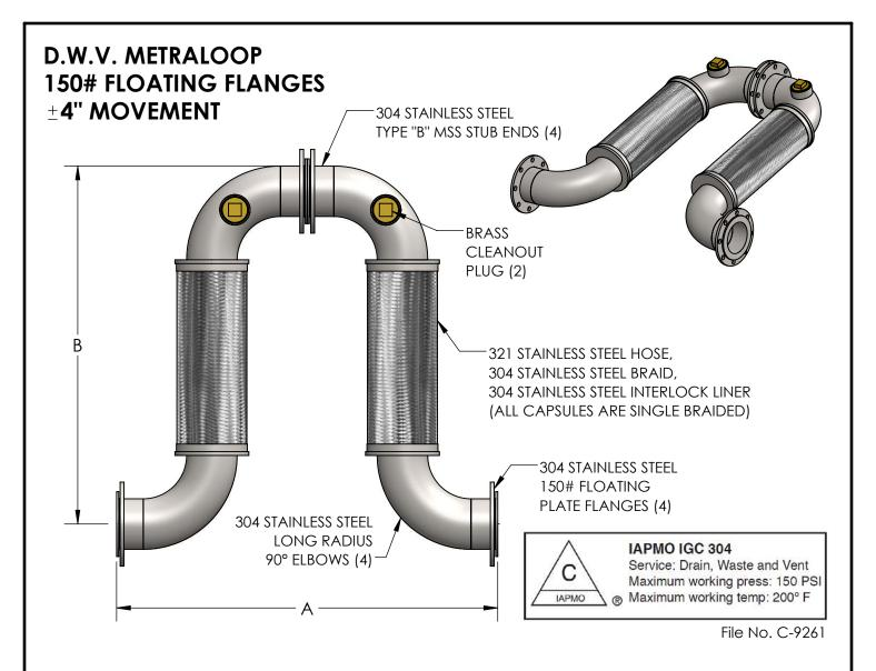
NOTE: D.W.V. METRALOOPS INSTALLED IN ANY ORIENTATION OTHER THAN HANGING DOWN MUST HAVE THE 180° RETURN SUPPORTED. (SEE INSTALLATION INSTRUCTIONS.)
