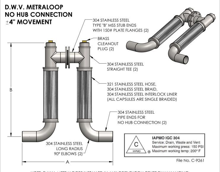
NOTE: D.W.V. METRALOOPS INSTALLED IN ANY ORIENTATION OTHER THAN HANGING DOWN <u>MUST</u> HAVE THE 180° RETURN SUPPORTED. (SEE INSTALLATION INSTRUCTIONS.)
