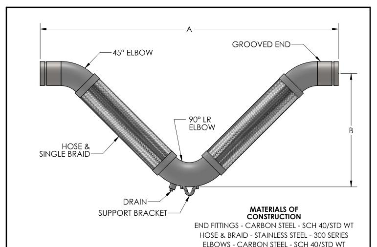
NOTE: V-LOOPS 2" AND LARGER INSTALLED IN ANY ORIENTATION OTHER THAN HANGING DOWN *MUST* HAVE THE 180° RETURN SUPPORTED. (SEE INSTALLATION INSTRUCTIONS.)
