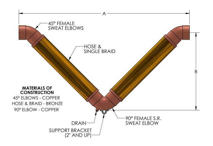
NOTE: V-LOOPS 2" AND LARGER INSTALLED IN ANY ORIENTATION OTHER THAN HANGING DOWN <u>MUST</u> HAVE THE 180° RETURN SUPPORTED. (SEE INSTALLATION INSTRUCTIONS.)
