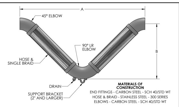
NOTE: V-LOOPS 2" AND LARGER INSTALLED IN ANY ORIENTATION OTHER THAN HANGING DOWN <u>MUST</u> HAVE THE 180° RETURN SUPPORTED. (SEE INSTALLATION INSTRUCTIONS.)
