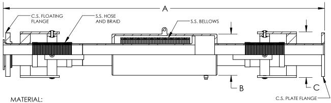
BELLOWS - MULTI-PLY STAINLESS STEEL HOSE AND BRAID - STAINLESS STEEL OTHER PARTS - CARBON STEEL
