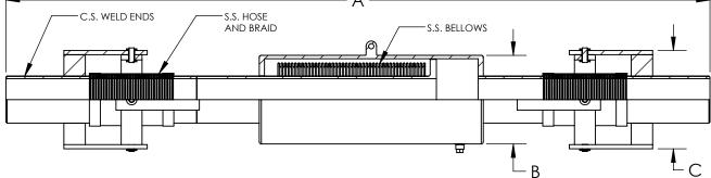
MATERIAL: BELLOWS - MULTI-PLY STAINLESS STEEL HOSE AND BRAID - STAINLESS STEEL OTHER PARTS - CARBON STEEL
