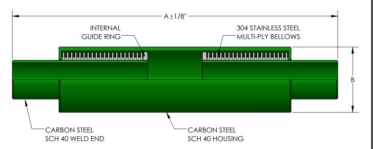
THIS EXPANSION JOINT IS DESGINED FOR AXIAL MOVEMENT ONLY. PIPE MUST BE PROPERLY GUIDED AND ANCHORED PER THE RECOMMENDATIONS OF THE EXPANSION JOINT MANUFACTURERS ASSOCIATION.
