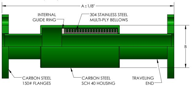
THIS EXPANSION JOINT IS DESGINED FOR AXIAL MOVEMENT ONLY. PIPE MUST BE PROPERLY GUIDED AND ANCHORED PER THE RECOMMENDATIONS OF THE EXPANSION JOINT MANUFACTURERS ASSOCIATION.
