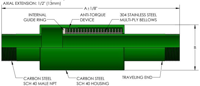
THIS EXPANSION JOINT IS DESGINED FOR AXIAL MOVEMENT ONLY. PIPE MUST BE PROPERLY GUIDED AND ANCHORED PER THE RECOMMENDATIONS OF THE EXPANSION JOINT MANUFACTURERS ASSOCIATION.
