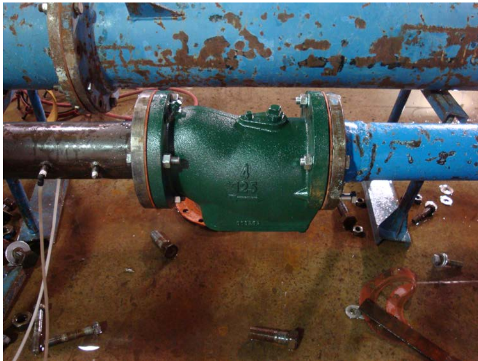
Figure 1. 4-inch strainer installation (Metraflex strainer shown).
