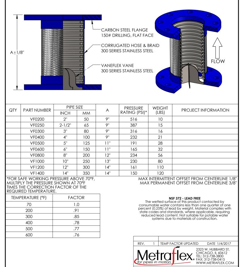
**MODEL VF** VANEFLEX WITH 150# PLATE FLANGES
