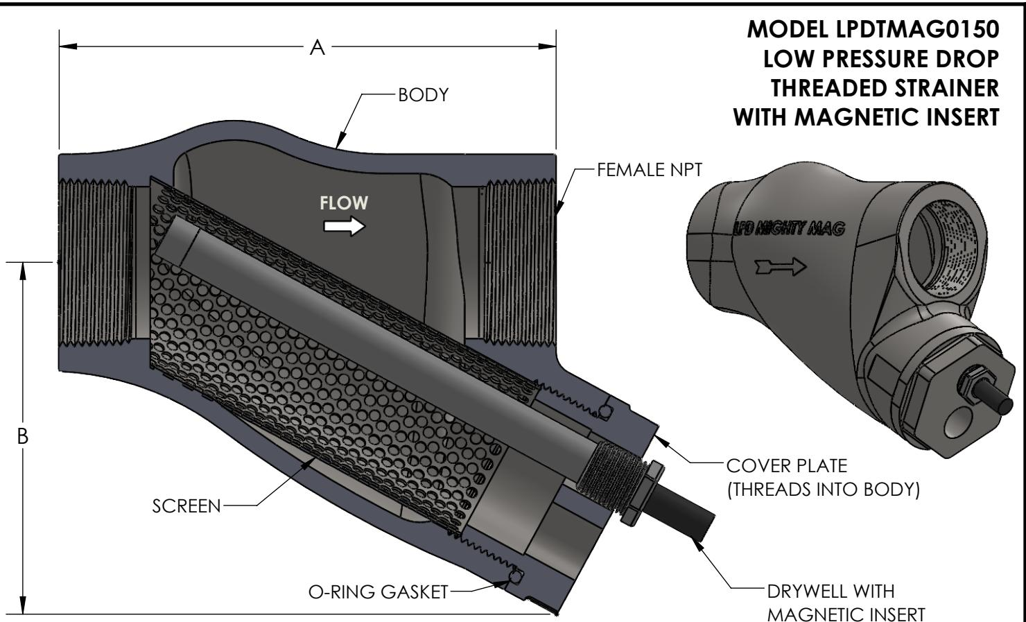
PRODUCT CAN BE ROTATED 90° AXIALLY TO PROVIDE MAINTENANCE CLEARANCE
